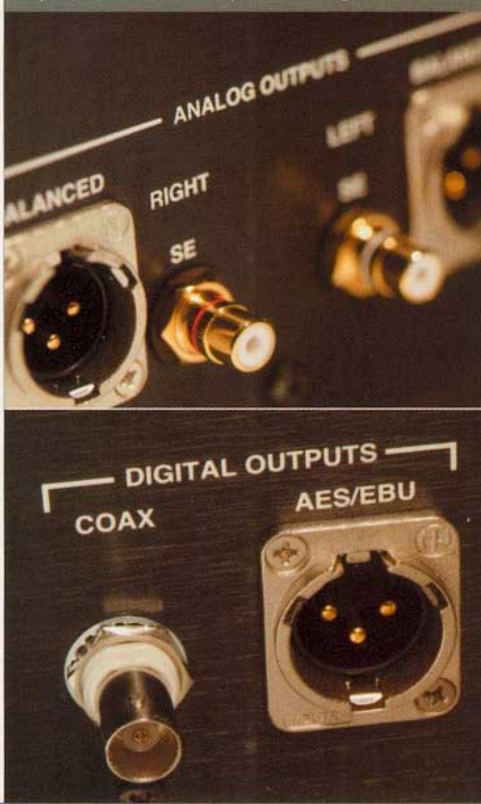
Below and left: balanced and unbalanced analogue outputs, and the same options for digital outs too
